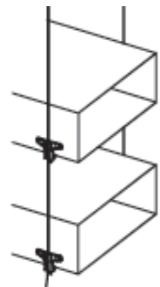
Rectangular Ductwork (double tier)
